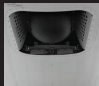
ABOVE: THE PC-12'S SURVEILLANCE POD RETRACTS, ALLOWING THE PLANE ANONYMITY ON THE RUNWAY.
