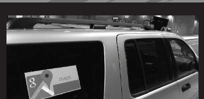
ABOVE: PHILLY P.D. S.U.V. WITH ELSAG MPH-9000 AND GOOGLE MAPS DECAL. PHOTO BY MATT BLAZE.
